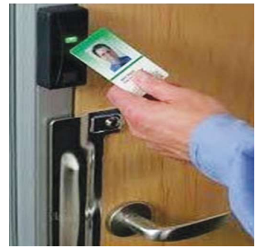
Fig. 3.8: Proximity card reader
